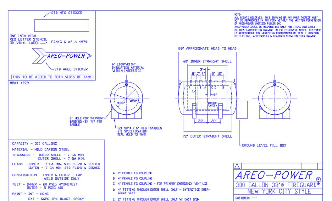
F 2' INTERNAL MONITOR INTERSTICE MONITOR PIPE WITH MALE NPT AT TOP
